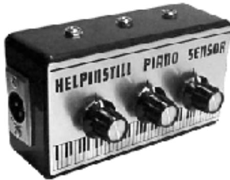
The control box is a passive unit. It does not require batteries, phantom power, or any other power source. This means it is compatible with sound systems worldwide, and requires no maintenance. The XLR connector provides an output at mic level, while the 1/4" jack high-impedance output is comparable to that of an electric guitar.
