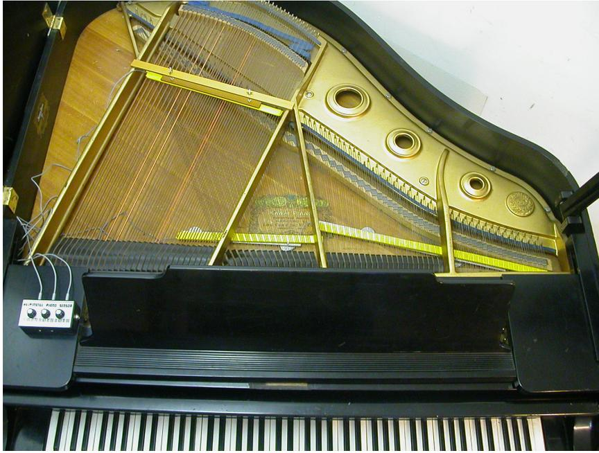
The silver support bars are used to support two sensors under the middle and treble strings. The gold double support bar suspends the third sensor over the bass strings. Before installing any of the pickup strips, remove the tie wraps from the cables and **smooth out, stretch and straighten the cables**. If they kink and curl under the strings, they may touch them and cause a buzzing noise.
